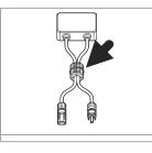
a) Installation of small suppressor on appliance power cord
