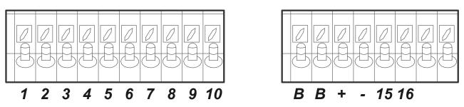
Inverter pinouts for sensors and accessories
