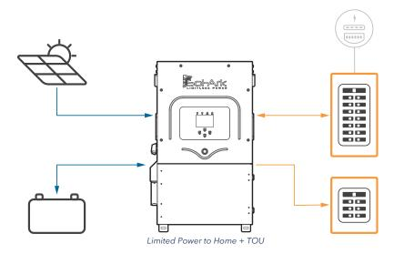
**Time:** Programable time intervals over a 24h period. All time slots **MUST** follow chronological order and must be programmed. **Power(W):** Sets the maximum discharge rate of the battery during the corresponding time slot.
