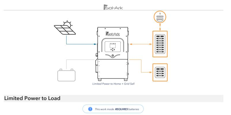
Limited Power to Load: This mode limits the solar production to cover "LOAD" demand (essential loads panel) exclusively. In this mode, the system disregards loads in the main service panel and will not deliver power to the "GRID" breaker.
