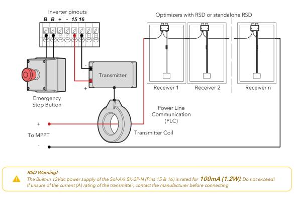
A transmitter that exceeds the maximum 100mA limit can still be integrated into the Sol-Ark inverter through an external power supply connected to the "LOAD" output. Pressing the e-stop button will disconnect all AC outputs, cutting power to the "LOAD" service panel which will initiate rapid shutdown.
