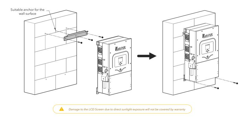
G. Mount the inverter in the optimal orientation as shown below.
